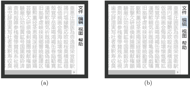
Fig. 5. The case of (simplified) Chinese: a shrink factor of 0.9 (b) seems more suitable than 0.8 (a) for the interface controls (here the main menu).
