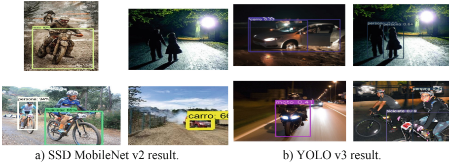
Fig. 6. Object detection result with SSD MobileNet v2 and Yolo V3
