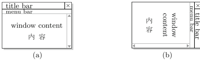
Fig. 1. A mock-up of a vertical right-to-left window chrome (a) matching a conventional window layout (b). The usage of a vertical script should be envisioned in place of the rotated English labels.
